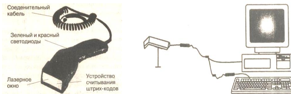
31-rasm. MS-951 qo‘lli skaner va uning personal kompyuterga ulanishi 7 .
