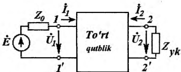
6.1-rasm. To'rtqutblikning shartli belgilanishi.
