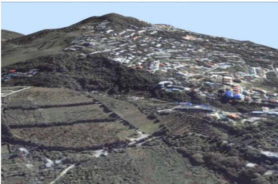
27-rasm. 3D modelini yaratish uchun DEM va Google rasmlarini birlashtirish
