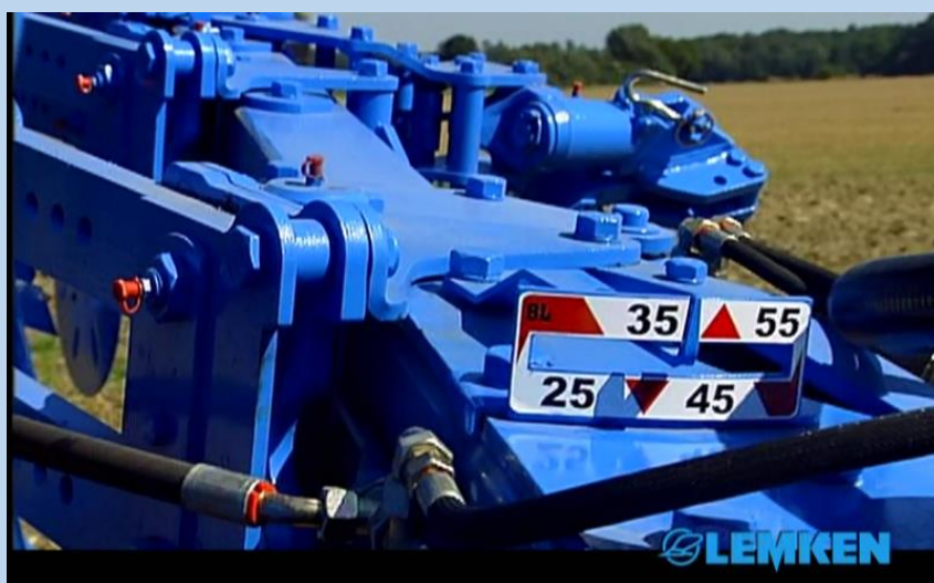
35-rasm. Lemken firmasi plugining qamrash kengligini o‘zgartirish innovatsion qurilmasi
