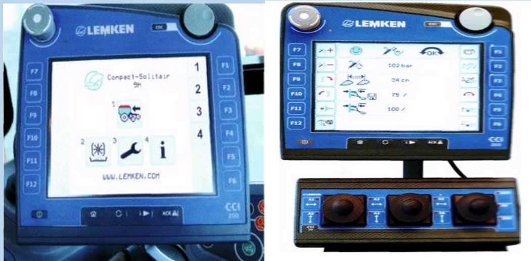
25-rasm. Belgilar va piktogramma qurilmasi (a) va plugni boshqarish uchun djoystli SSIISOBUS terminali (v)
