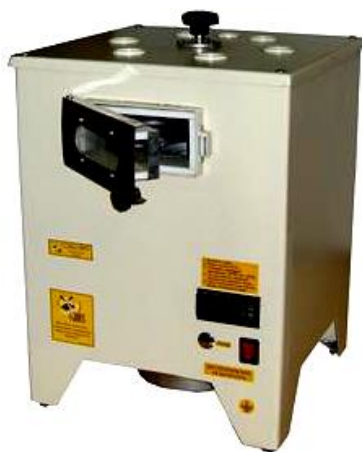
9-rasm. Quritish shkafi va hir xil o'lchamli alyumin byuks idishlar
